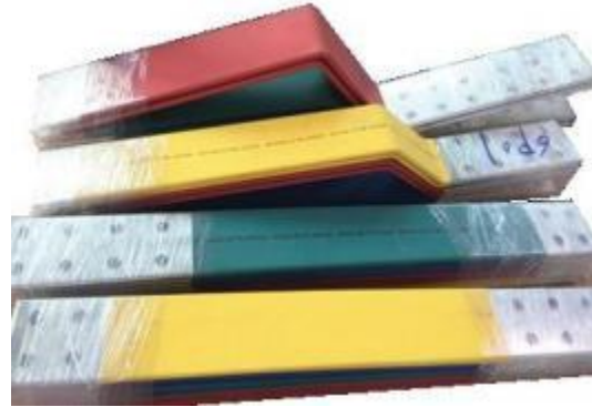
Hard connection (overlapping copper bars)
